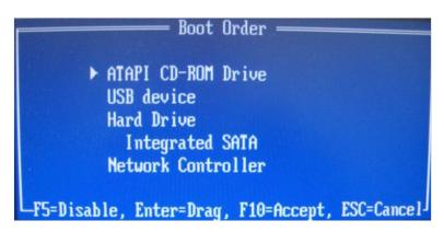
Restart the computer. While the system is restarting, run the system setup program (BIOS). The BIOS can be activated by pressing a special key such as ESC, F1, F12 or DELETE. (Refer to your system manufacturer's documentation for the correct key.)
