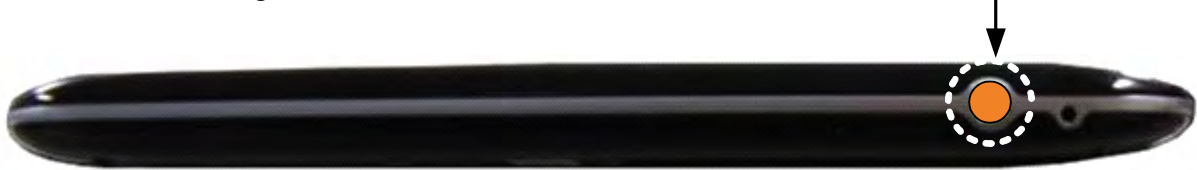
Figure 6.2 – Power LED, Orange
