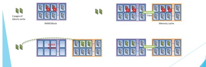
With Trim, the operating system tells the disk it is trimming away the blocks. In the background, the SSD can copy the data and remove the blocks in its own time. Unlike the previous scenario, the pages are not overwritten at that time, so those pages are available for a future write operation. This maximizes SSD performance.
