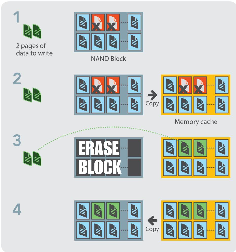
Figure 2: The process of overwriting data
