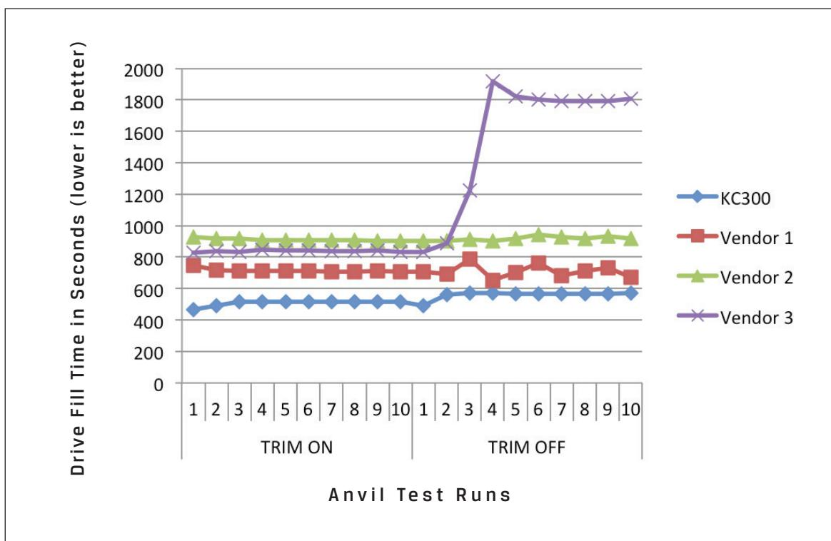
The bottom axis shows the number of Anvil runs from Run #1 to Run #10, first with TRIM On, then with TRIM Off.
