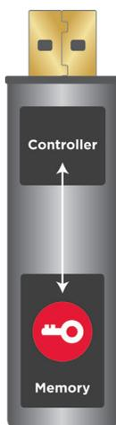
**Figure 1.** Drives that store encryption keys in the clear make it easier for hackers to read the key and steal the data stored on the device.
