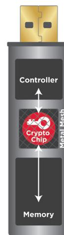
**Figure 2.** Drives that store encryption keys in a separate tamper-resistant cryptochip module are significantly more difficult to compromise. They tend to feature unique defenses, such as a metal mesh cladding and self-destruct function in case of physical attacks.
