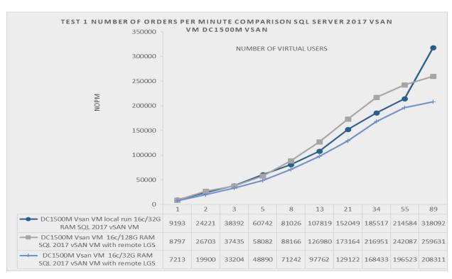
Figure 2.3 Test 1a,b,c: DC1500M vSAN datastore NOPM comparison different DRAM size
