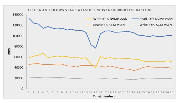
Figure 6.4 Test 5a and 5b Noisy neighbour IOPS, DC1500M NVMe and Micron 5200 eco vSAN datastore
