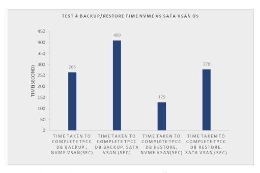
Figure 5.6 Time taken to complete SQL Server 2017 TPCC DB backup/restore operation Micron 5200 eco SATA and DC1500M NVMe SSD vSAN datastore(sec)
