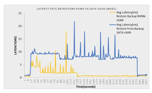
Figure 5.5 Latency(ms) comparison SQL Server 2017 TPCC DB Restore Micron 5200 eco SATA and DC1500M NVMe SSD vSAN datastore
