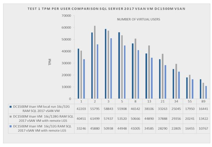
Figure 2.4 Test 1a,b,c: DC1500M vSAN datastore TPM comparison different DRAM size
