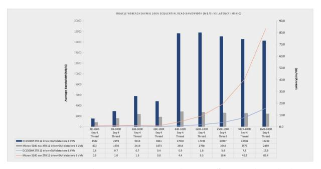
Figure 1.4 DC1500M vSAN datastore vs Micron 5200 eco vSAN datastore, 100R/OW, sequential, QD=8, threads=4, HCIBench 6 VMs read throughput(MB/s) and average read latency(ms/IO)
