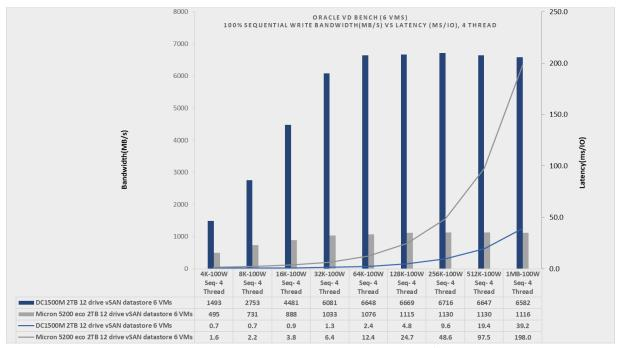
Figure 1.5 DC1500M vSAN datastore vs Micron 5200 eco vSAN datastore, 100W/OR, sequential, QD=8, threads=4, HClBench 6 VMs read throughput(MB/s) and average read latency(ms/IO)
