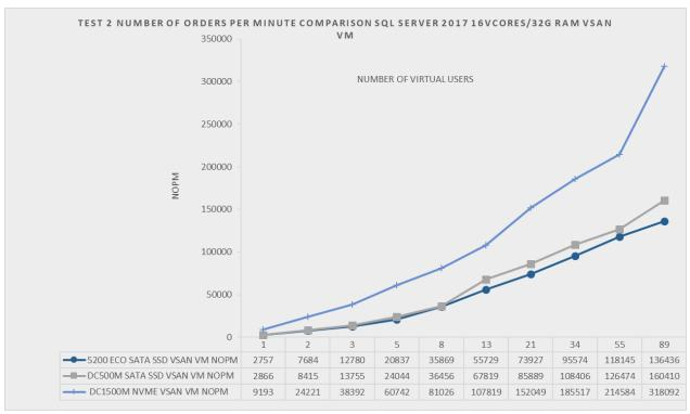
Figure 3.3 Test 2: NOPM comparison NVME vs SATA VSAN datastore
