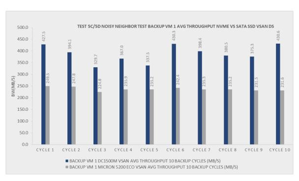
Figure 6.10 Test 5C/5D Backup VM throughput, noisy neighbour implementation NVMe vs SATA SSD vSAN datastore
