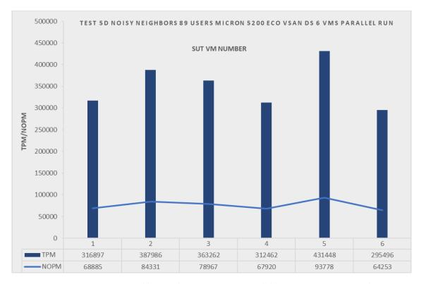
Figure 6.7 Test 5D TPM, noisy neighbour implementation six VM parallel run Micron 5200 eco vSAN datastore
