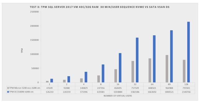
Figure 4.2 Test 3 TPM comparison SQL Server 2017 DB stress test on Micron 5200 eco SATA and DC1500M NVMe SSD vSAN datastore
