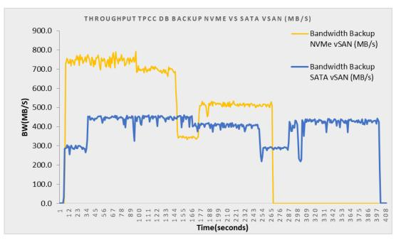
Figure 5.2 Throughput comparison SQL Server 2017 TPCC DB Backup Micron 5200 eco SATA and DC1500M NVMe SSD vSAN datastore(MB/s)
