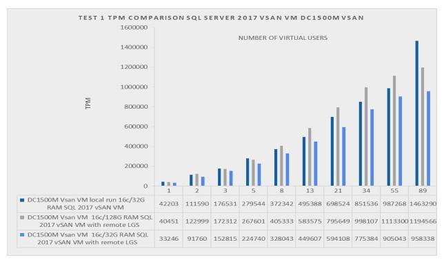
Figure 2.2 Test 1a,b,c: DC1500M vSAN datastore TPM comparison different DRAM size
