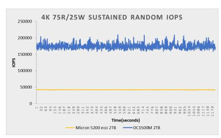
Figure a) Second-by-second IOPS comparison of DC1500M 1920G and Micron 5200 ECO 1920G SATA SSD. Tested on a single physical drive attached as a secondary to a Linux system with foo v3.17 once the SSDs have reached a steady state of performance. Based on a block size of 4k, read percentage of 75% and a queue depth of 32
