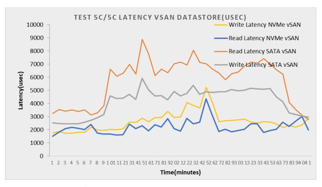
Figure 6.9 Test 5C/5D Latency, noisy neighbour implementation NVMe vs SATA SSD vSAN datastore
