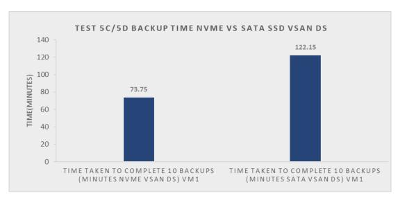
Figure 6.11 Test 5C/5D Backup VM time taken to complete backup, 10 cycles noisy neighbour implementation NVMe vs SATA SSD vSAN datastore
