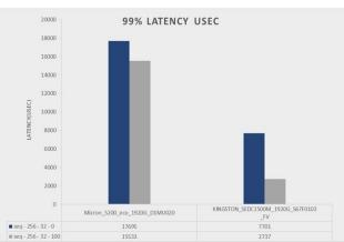
Figure b) Sequential BW(MB/s) read/write and latency(usec) comparison of DC1500M 1920G and Micron 5200 ECO 1920G SATA SSD. Tested on a single physical drive attached as a secondary to a Linux system with foo v3.17 once the SSDs have reached a steady state of performance. Based on a block size of 256k and a queue depth of 32
