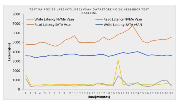
Figure 6.5 Test 5a and 5b Noisy neighbour latency, DC1500M NVMe and Micron 5200 eco vSAN datastore
