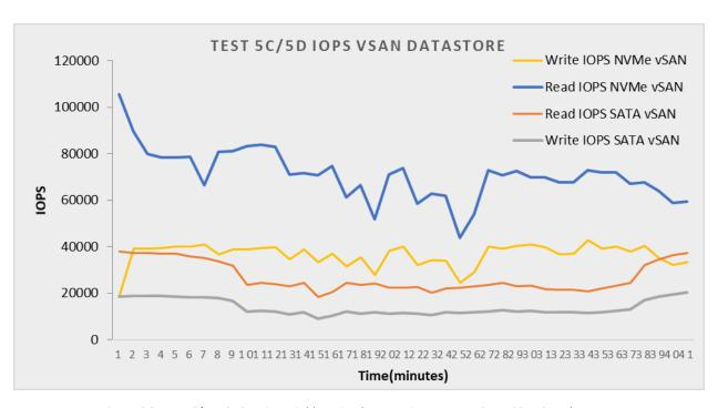
Figure 6.8 Test 5C/5D IOPS, noisy neighbour implementation NVMe vs SATA SSD vSAN datastore
