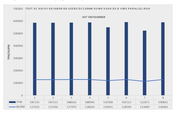
Figure 6.6 Test 5c TPM, noisy neighbour implementation eight VM parallel run DC1500M NVMe vSAN datastore
