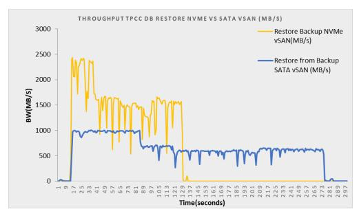
Figure 5.4 Throughput comparison SQL Server 2017 TPCC DB Restore Micron 5200 eco SATA and DC1500M NVMe SSD vSAN datastore(MB/s)
