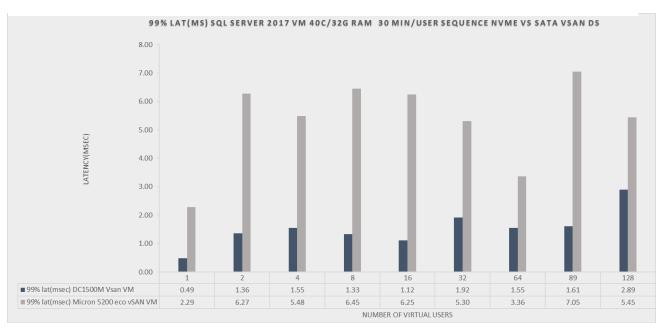
Figure 4.5 Test 3 99<sup>th</sup> % latency(ms) comparison SQL Server 2017 DB stress test on Micron 5200 eco SATA and DC1500M NVMe SSD vSAN datastore
