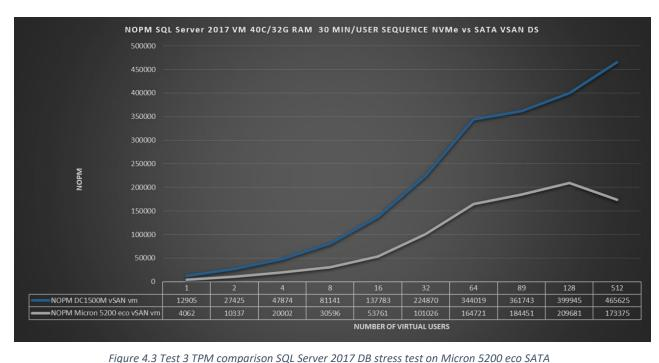
rigure 4.3 Test 3 TPM comparison SQL Server 2017 DB stress test on Micron 5200 eco SATA and DC1500M NVMe SSD vSAN datastore
