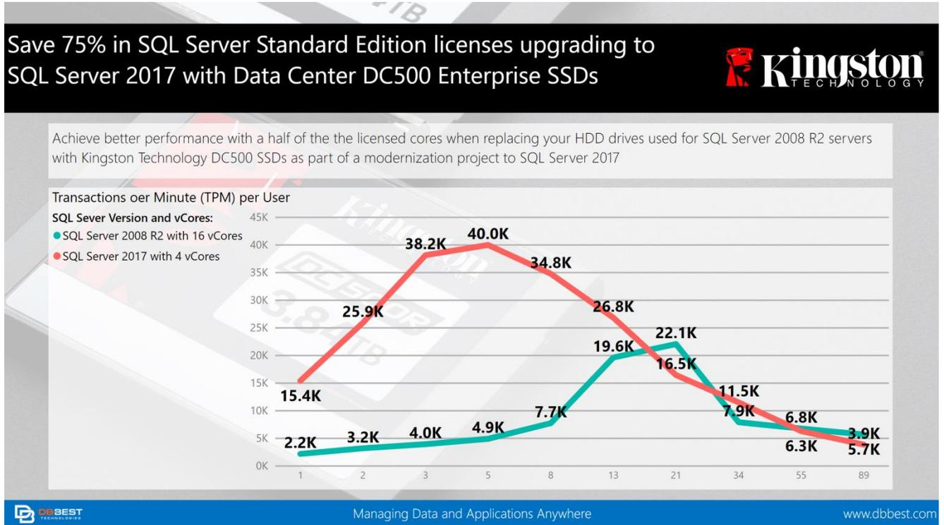
Based on prior benchmarking performed with other hardware manufacturers and cloud vendors, we had a good idea that moving from older versions of SQL Server to SQL Server 2017 using SSD for data log and tempdb could use fewer vCores.
