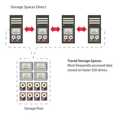
Storage Spaces Direct requires a minimum of four storage nodes, and in addition to fault tolerance and high availability, it provides tiered storage and deduplication functionality.
