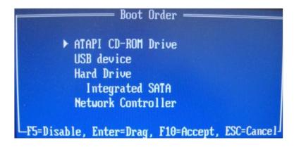
Restart the computer. While the system is restarting, run the system setup program (BIOS). The BIOS can be activated by pressing a special key such as ESC, F1, F12 or DELETE. (Refer to your system manufacturer's documentation for the correct key.)
